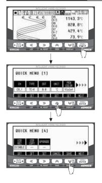
Press the ENTER key once in RUN mode and it enters to QUICK MENU. QUICK MENU consists of usually used parameters for quickly parameter setting.
